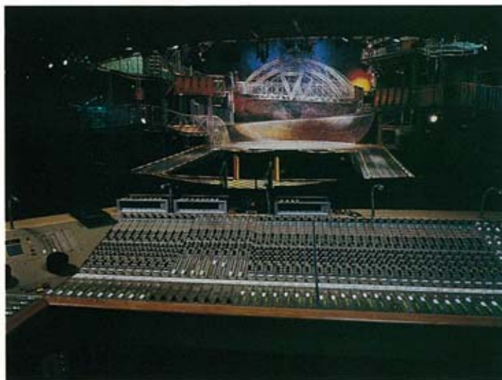
Clive Green & Co's 48-channel Cadac sound console, now in its ninth year mixing the successful musical Starlight Express . The Cadac was the first theatre sound console in the West End to feature computer control.
