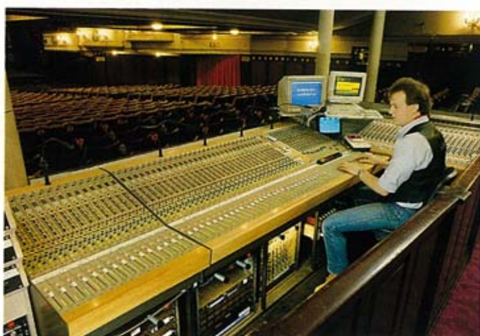
One of the largest Cadac E-type mixing consoles in use on 'Miss Saigon' in London. Clive Green & Co's E-type system provides a total of 86 inputs to handle the sound of the 41-strong cast, the elaborate sound effects and 30 musicians.
