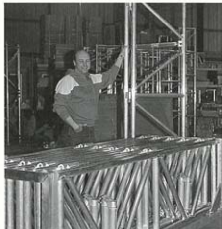
Chris Cronin with Total Fabrication's latest folding truss designed to provide a combination of high load capacity with immense space saving. It can support over two tonnes across a 40 feet span and pack into less than 20% of the space required to house any conventional truss with similar load range. Sections come in eight feet lengths as standard and are designed to pack in groups of five.
